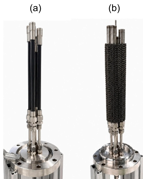
Fig. 5. (a) Assembly of four tubular CMS membranes connected to the reactor flange, (b) with POCS catalyst structures fitted over the membrane tubes.
