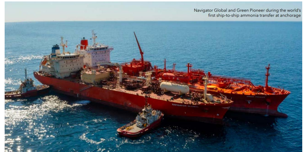
Photo of first vessel-to-vessel ammonia bunkering operation
