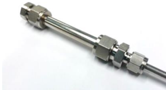
1.3 \mu\text{m} thick Pd-Ag membrane
