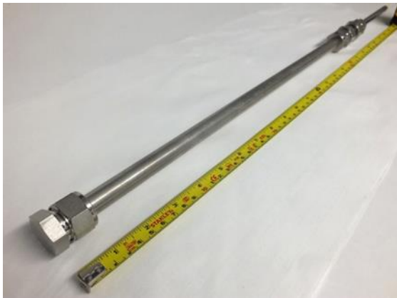
Ceramic supported thin Pd-based membranes (with Swagelok-graphite connectors)
