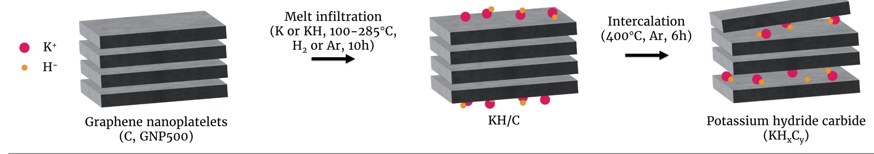
Synthesis: degree of intercalation With increasing melt infiltration and intercalation the temperatures diffraction peaks attributed to the KH<sub>x</sub>C<sub>y</sub> phase appear more intensely.
